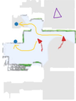
Fig. 4. APF Resistance Force. APF achieves cooperation by introducing resistance force among agents. In above situation, the yellow lines demonstrate agents' paths to their corresponding global goal. Due to the resistance force, the agent on the left is forced to choose a sub-optimal global goal instead of frontiers in the more promising part indicated by the purple triangle.
