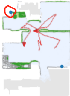
Fig. 2. Faulty Estimation of Value. In the above situation, Utility selects a cell at the corner of the room as a global goal since it's nearby space is unexplored. However, with prior knowledge about building structures, one should infer that such point should not be chosen.
