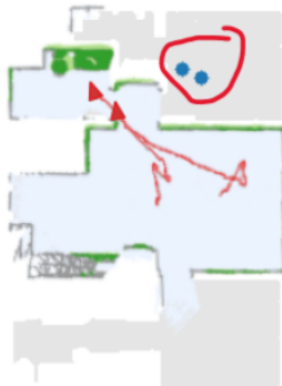
Fig. 3. Poor Cooperation. RRT performs planning independently, it's possible that agents choose close frontiers as goals, leading to duplicated exploration.
