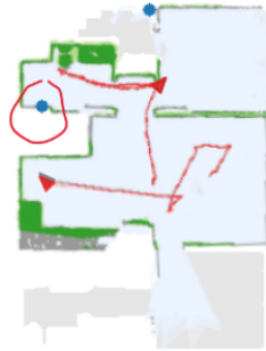
Fig. 1. Sensitive to Realistic Noise. Utility, Nearest, APF and the voronoi-based method performs cell-level goal searching, the above picture demonstrates a case when the agent selects a cell that is estimated as "unexplored" because of mapping error.
