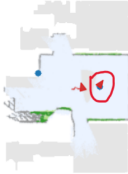
Fig. 5. WMA-RRT Locking Mechanism. In WMA-RRT, agents cooperatively maintain a tree and use a locking mechanism to avoid duplicated exploration. The above picture shows a case where agent on the right has to stay where it is since the path is locked by another agent.
